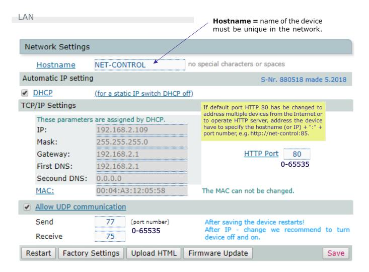
**MAC** must be unique in the network and must not be changed. The last three pairs of digits form the serial number.
